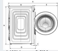
A: 1001.4 mm B: 518.8 mm C: 27.5 mm D: 512.3 mm E: 455.6 mm H: 845 mm
